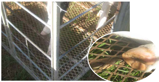
floor covered with metal grid
