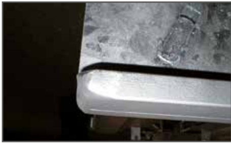
bearing surface of side skid is rounded off
