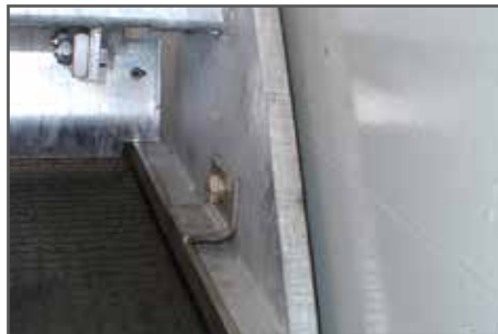
wide and bent up side skids, screwed on
