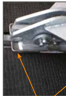
wide bearing for the center bracket, bent up in skid form
