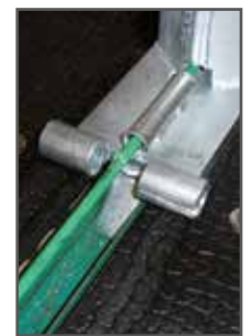
wide bearing for center bracket, welded on rod iron
