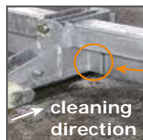
cleaning flap back stop: no contact to the surface
