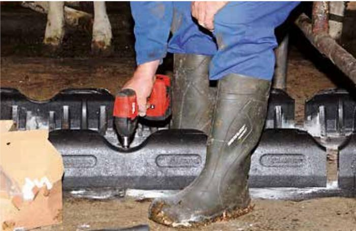
The rubber is available in lengths of 115 and 120 cm. At 18.5 cm it is higher than the maxiBOARD brisket board. But the rubber is softer and the incorporated rounded indentations are advantageous for positioning the front legs and head when lying down.
