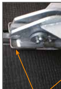
wide bearing for the center bracket, bent up in skid form
