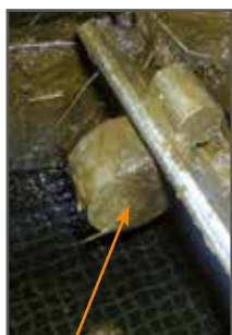
guiding skid on main cleaning flap
