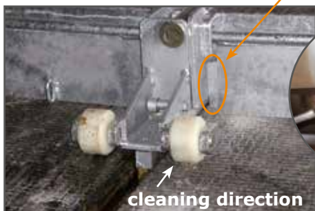
center bracket rests on wide plastic rollers
