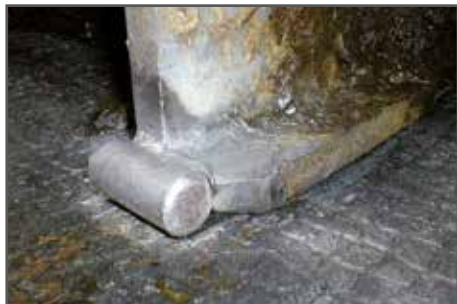
side skids with rod iron and wide bearing
