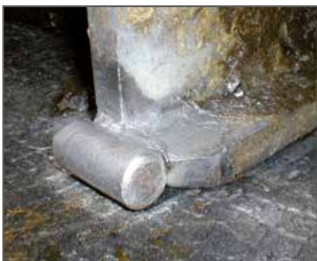
side skids with rod iron and wide bearing
