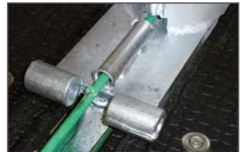
wide bearing for center bracket, welded on rod iron
