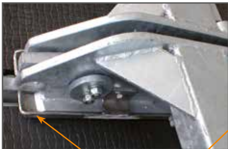
wide bearing for the center bracket, bent up in skid form
